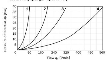
▼ Pressure differential  $\Delta p$  in relation to flow  $q_{v}$ , measured via the check valve: A → B
